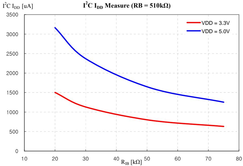
I<sup>2</sup>C Block operation current consumption curve
