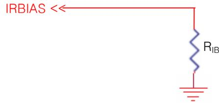
The R<sub>IB</sub> is only charged in making the I<sup>2</sup>C internal clock and should be implemented as above figure. The smaller R<sub>IB</sub> will increase the I<sup>2</sup>C internal clock frequency and current consumption. (Refer to the following consumption curve)
